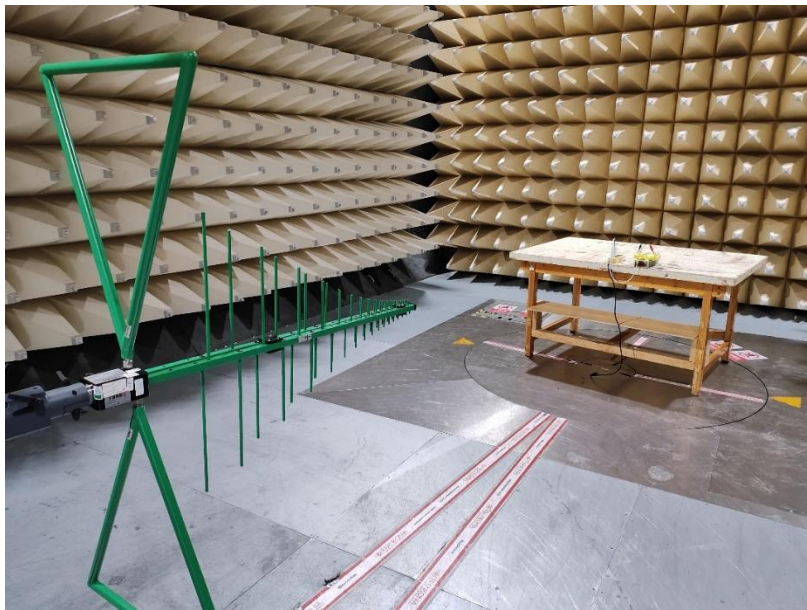
Photograph 3: Set-up for measurement of radiated emission
