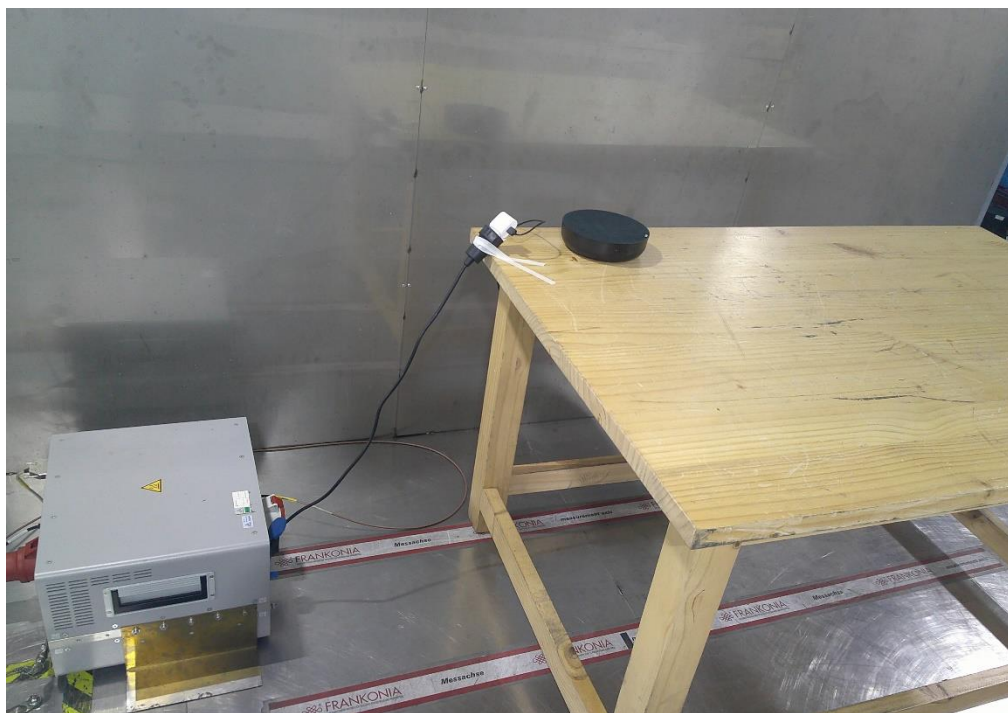
Photograph 2: Set-up photo for Conducted Emission
