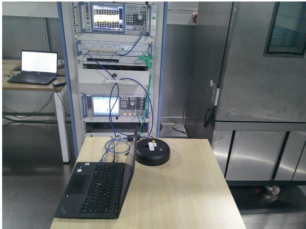
Photograph 1: Set-up photo for RF Conducted Test
