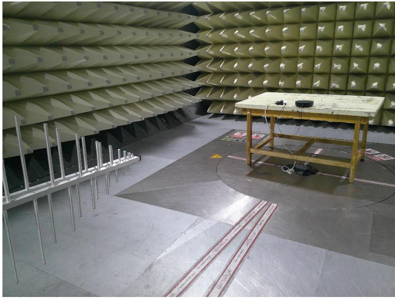
Photograph 3: Set-up for measurement of radiated emission
