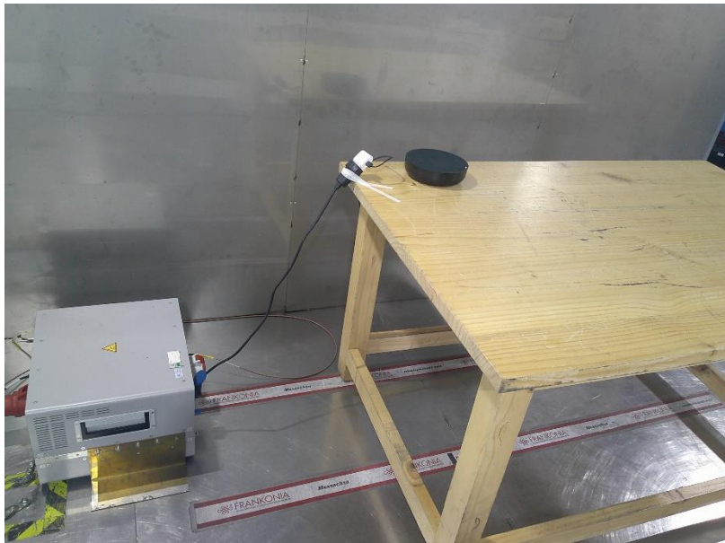
Photograph 2: Set-up for measurement of conducted emission
