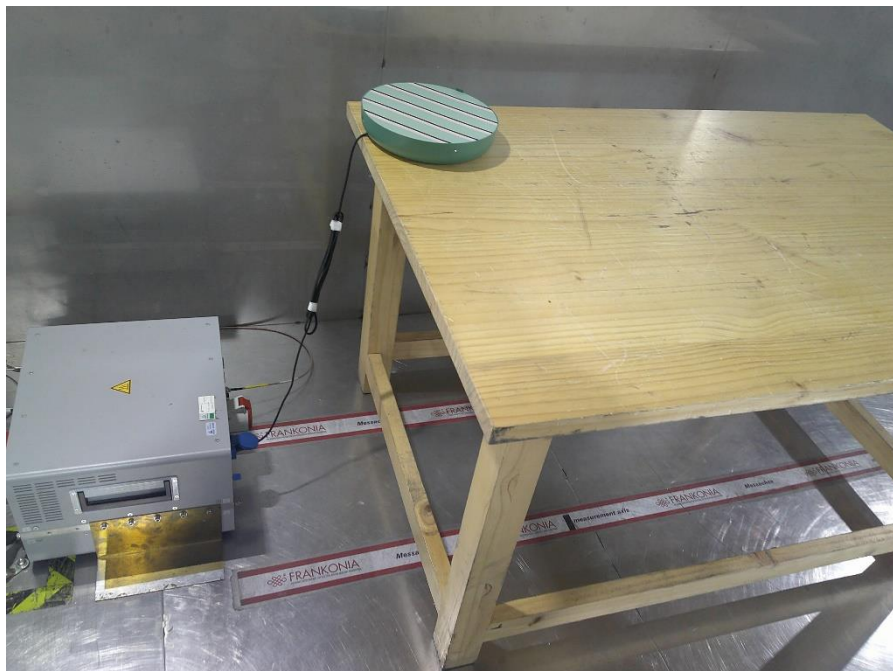
Photograph 2: Set-up for measurement of conducted emission
