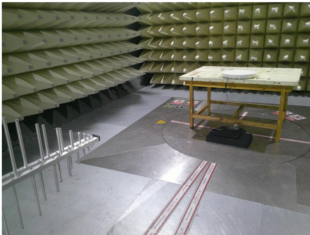
Photograph 3: Set-up photo for Radiated Emission, 30MHz - 1GHz
