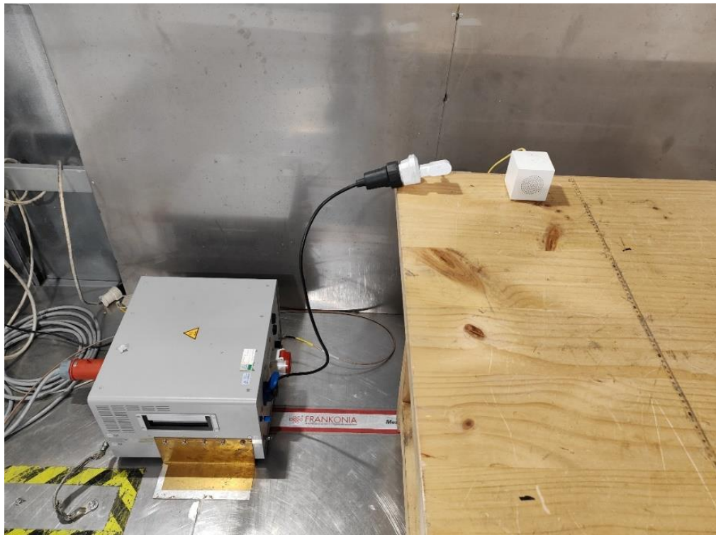
Photograph 2: Set-up photo for Conducted Emission
