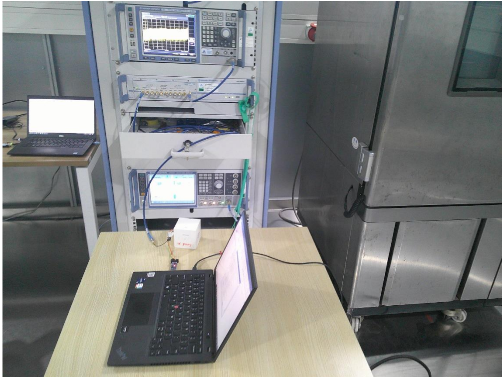
Photograph 1: Set-up photo for RF Conducted Test
