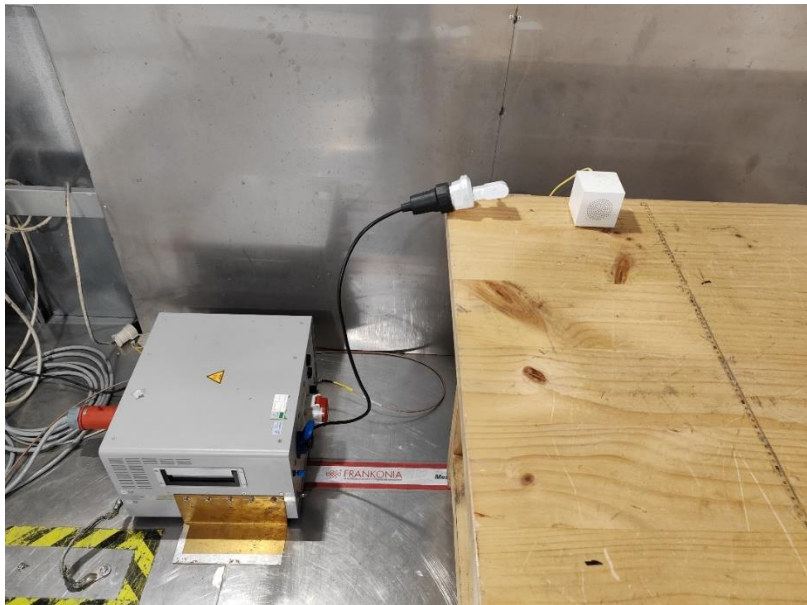
Photograph 2: Set-up for measurement of conducted emission
