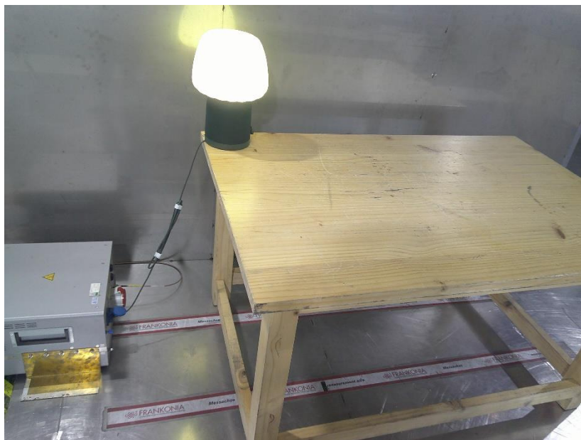
Photograph 2: Set-up for measurement of conducted emission
