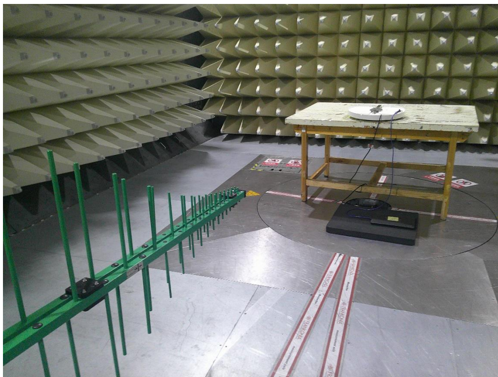
Photograph 3: Set-up photo for Radiated Emission, 30MHz - 1GHz
