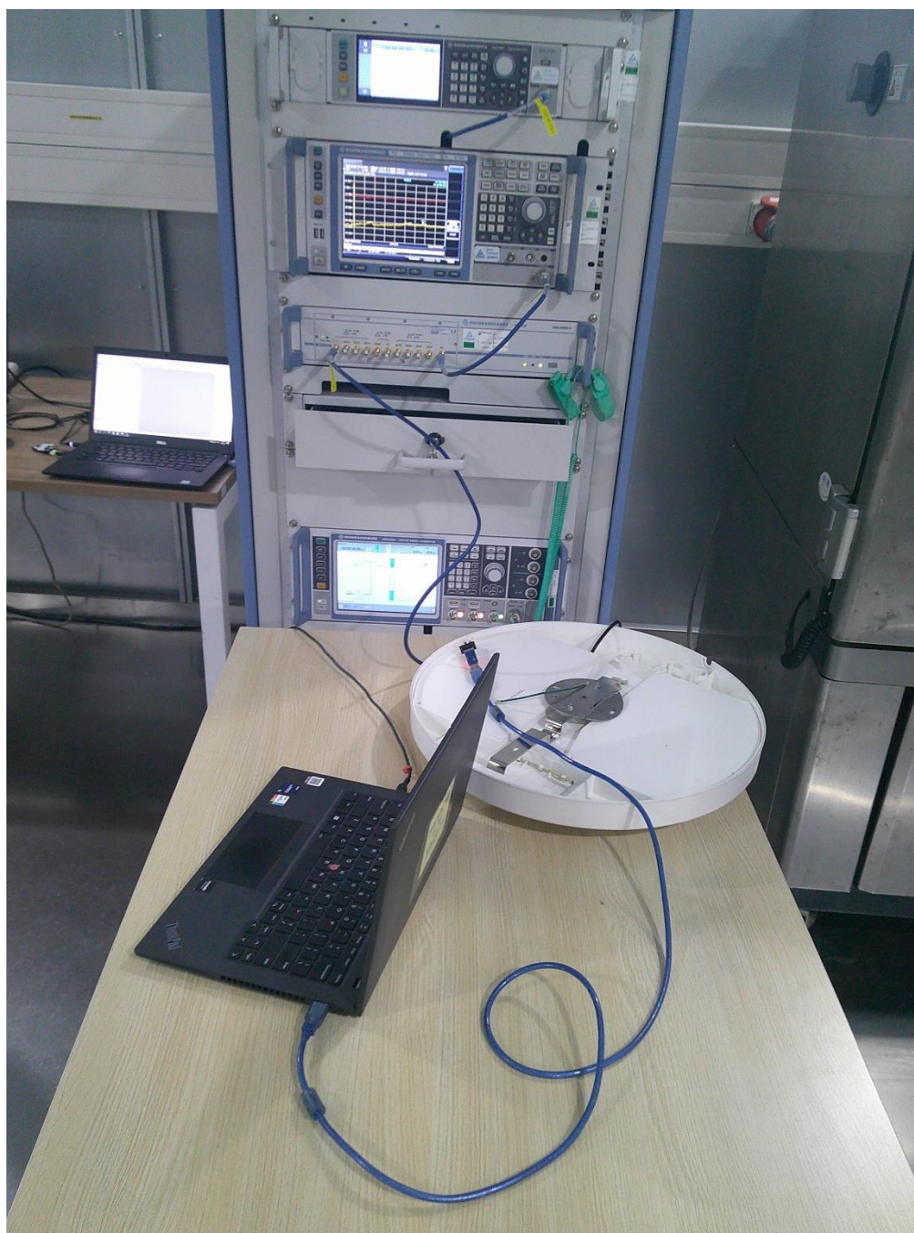
Photograph 1: Set-up photo for RF Conducted Test
