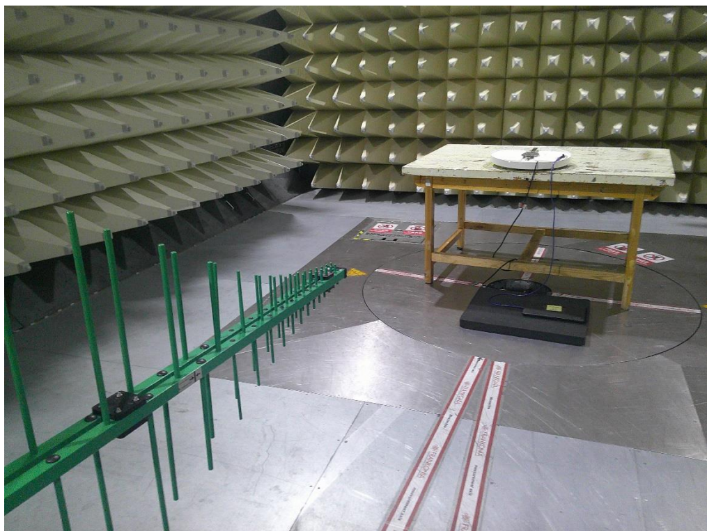
Photograph 3: Set-up photo for Radiated Emission, 30MHz - 1GHz
