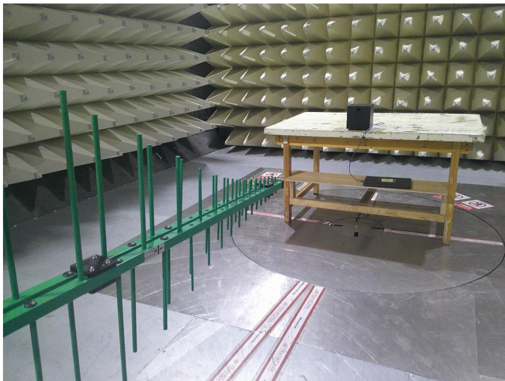
Photograph 3: Set-up photo for Radiated Emission, 30MHz - 1GHz
