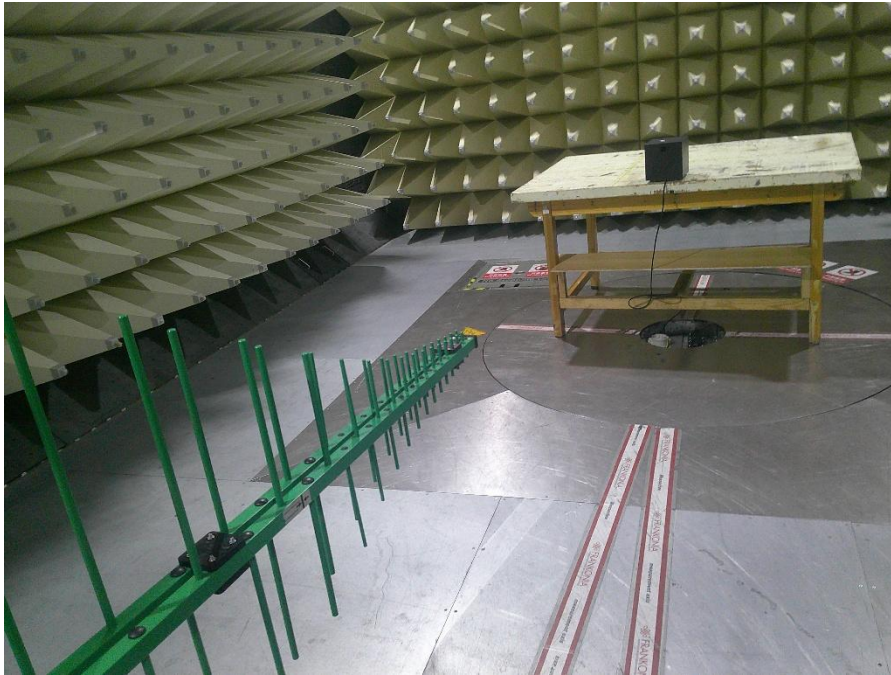
Photograph 3: Set-up for measurement of radiated emission
