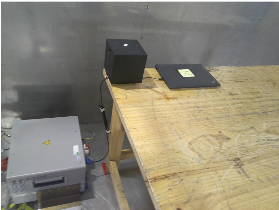
Photograph 2: Set-up for measurement of conducted emission
