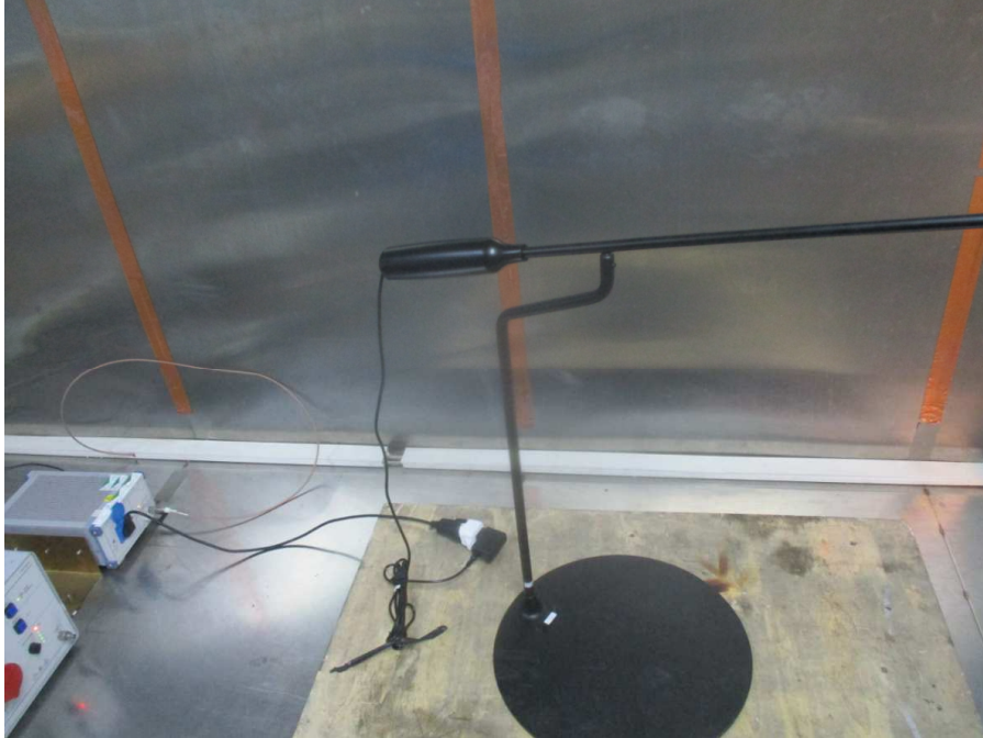
Photograph 1: Set-up for measurement of conducted emission
