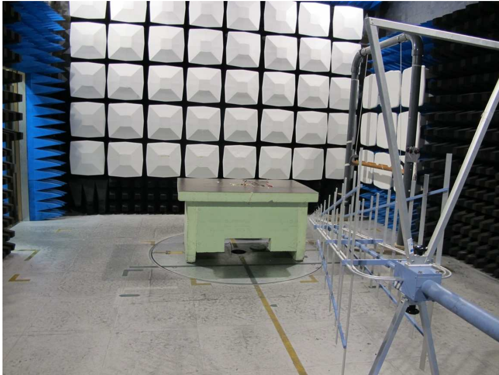
Test set up radiated emission 30 MHz – 1GHz
