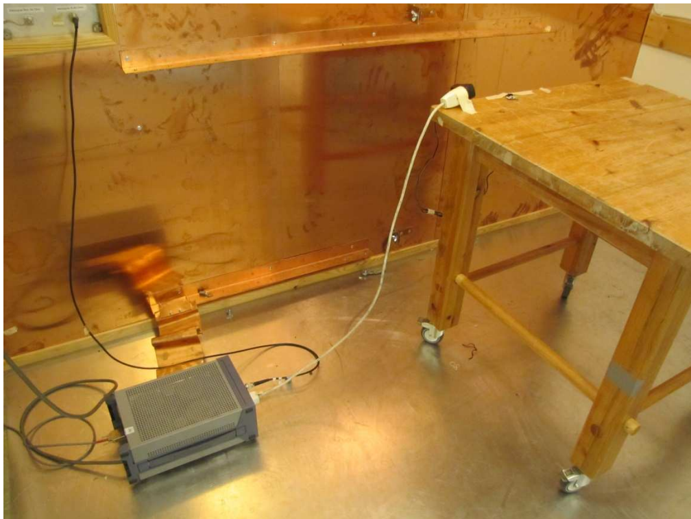
Test set up conducted emission 9 kHz – 30 MHz
