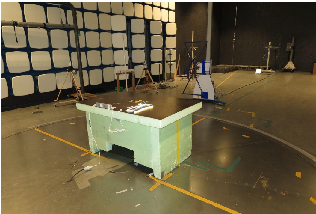
Test set up radiated emission 30 MHz – 1 GHz
