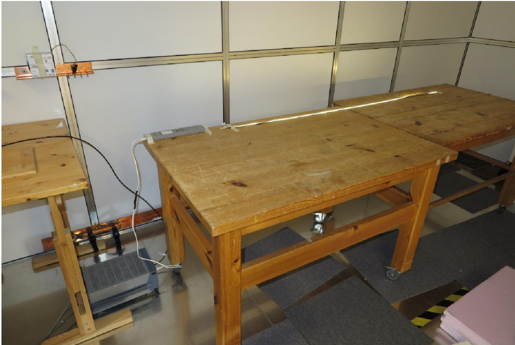
Test setup for conducted emission 150 kHz – 30 MHz
