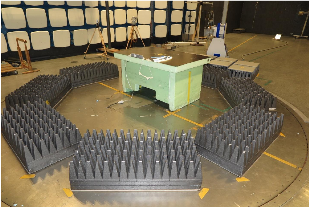
Test set up radiated emission 1 GHz – 13 GHz
