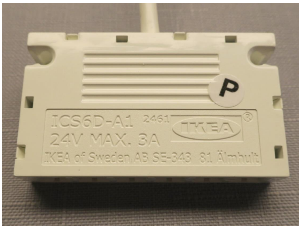
Photo 12 - External view of connector hub for the Optional output cord-set
