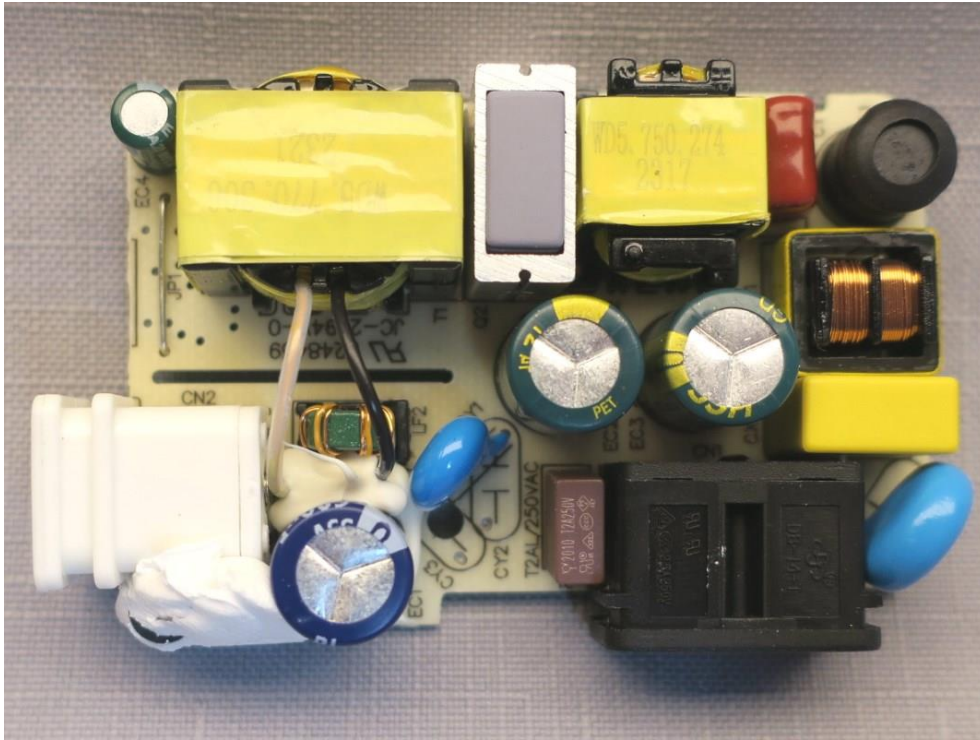
Photo 9 - View of the PWB component side, of ICPSW24-19-3
