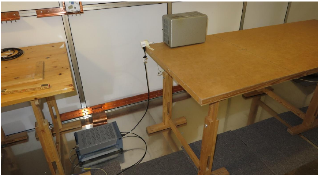
Test set up conducted emission 0.15 MHz – 30 MHz
