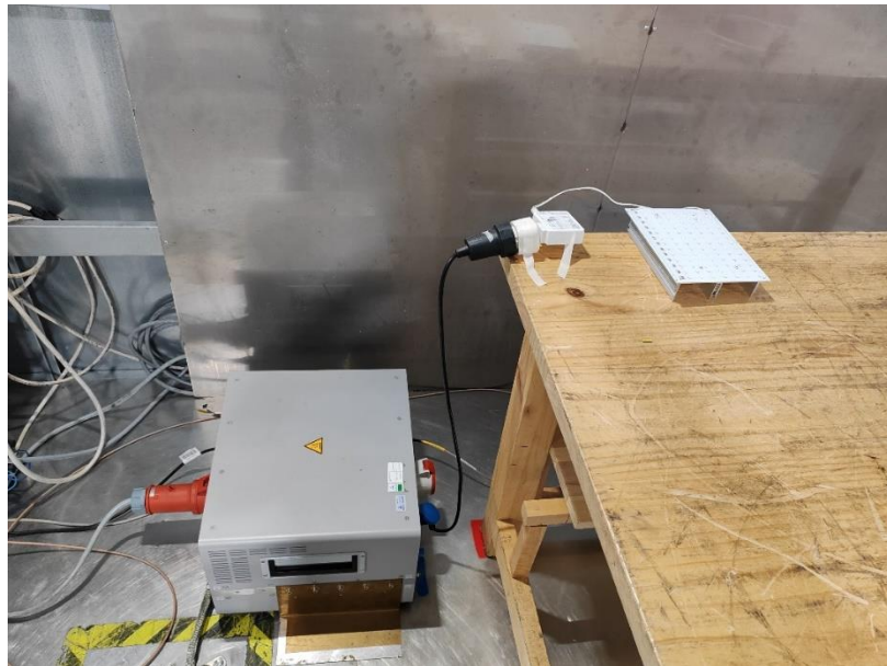
Photograph 2: Set-up for measurement of conducted emission
