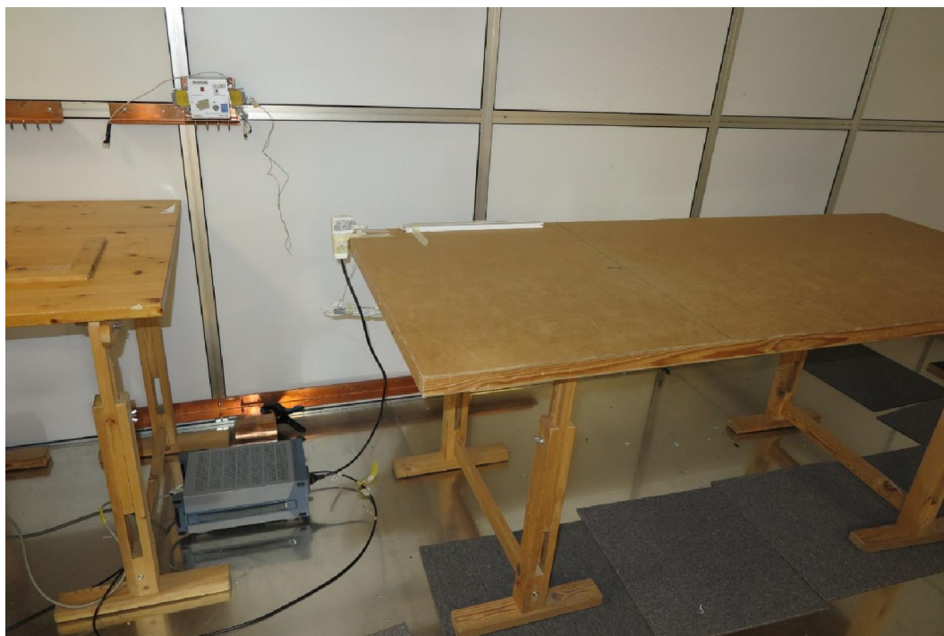
Test setup for conducted emission 150 kHz – 30 MHz
