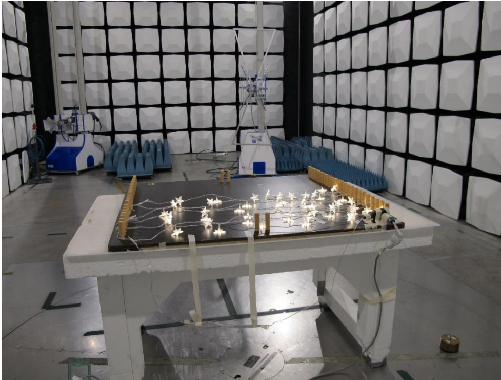
Test set up radiated emission 30 MHz – 1 GHz
