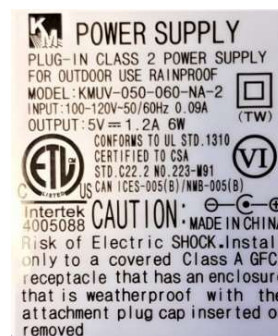
Photo of LED driver rating plate
