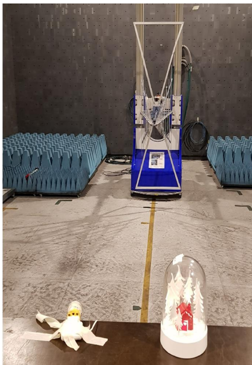
Test set up radiated emission 30 MHz – 1 GHz, 3 m
