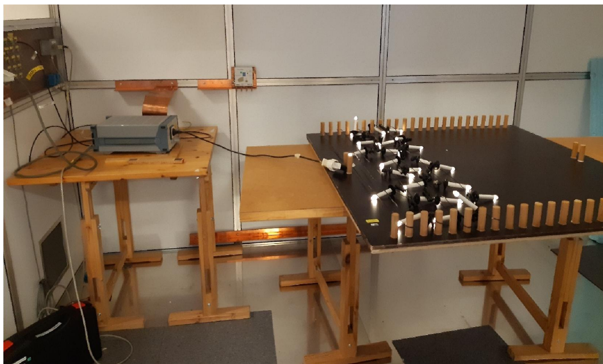
Test setup for conducted emission 150 kHz – 30 MHz
