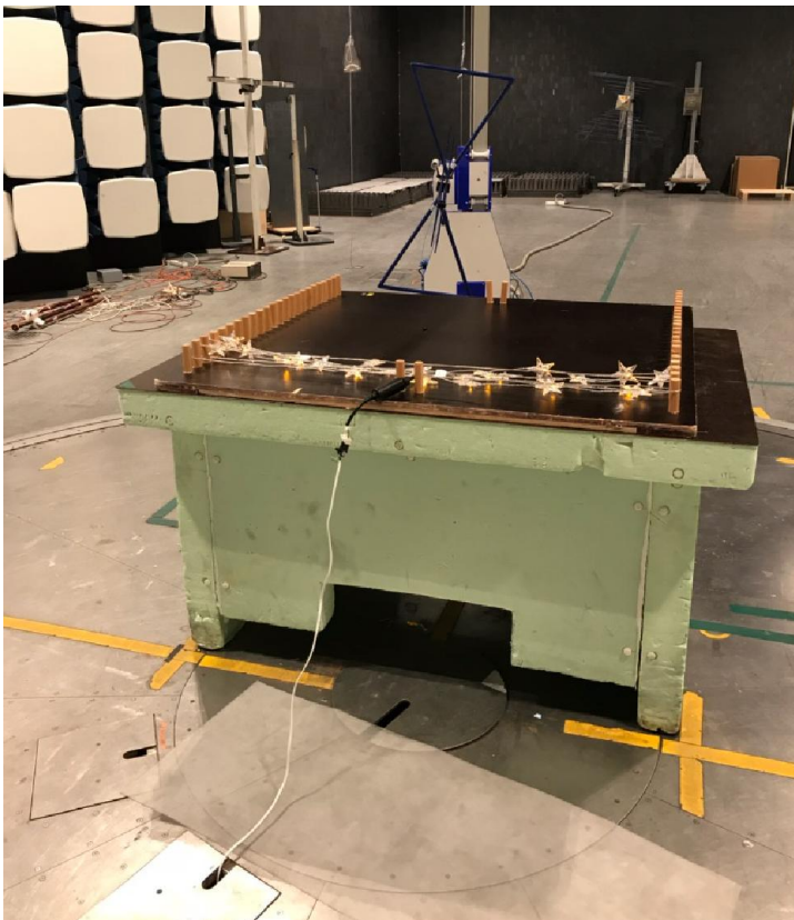
Test set up radiated emission 30 MHz – 1 GHz
