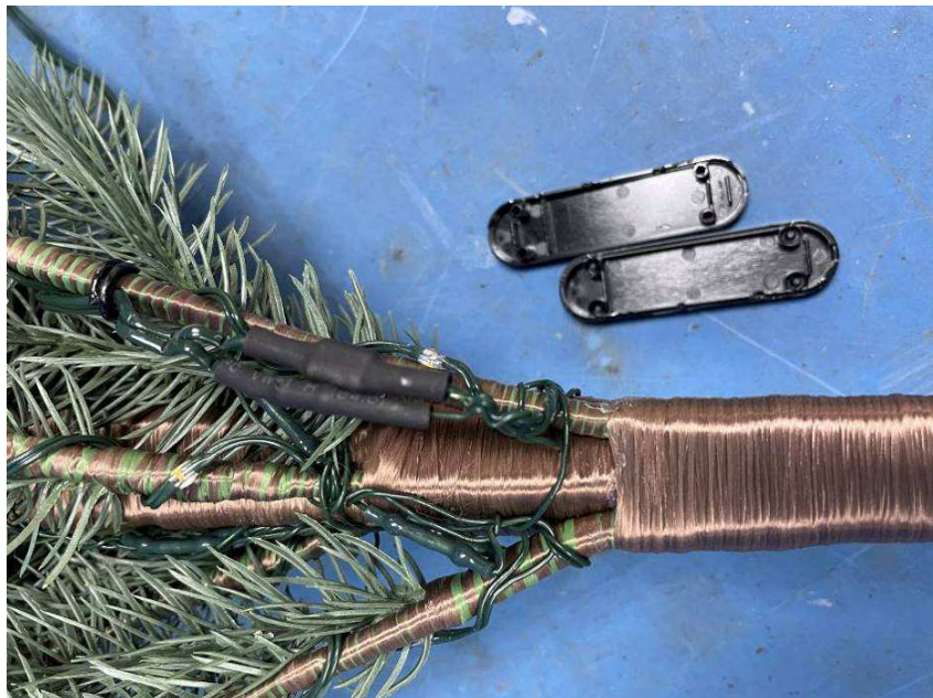
Internal view of conjunction box
