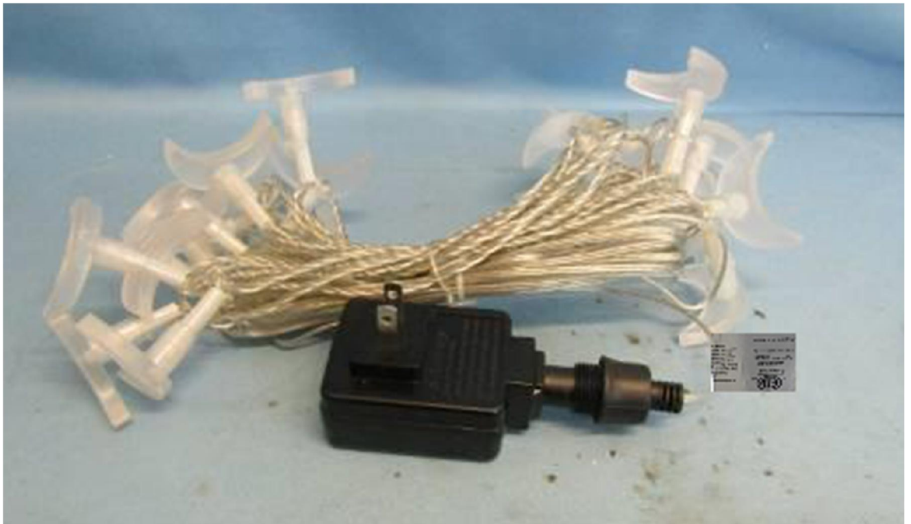
Label sticking on cable near the DC input of light chain
