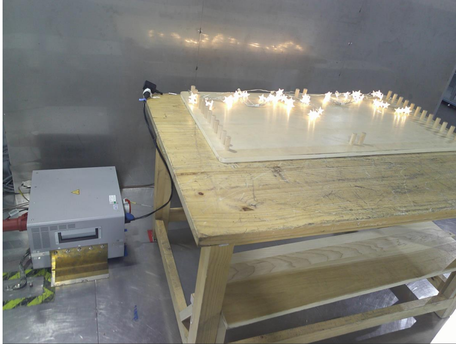
Photograph 1: Set-up for measurement of conducted emission
