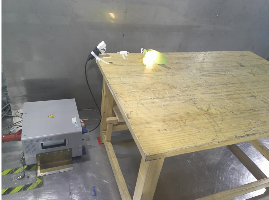
Photograph 1: Set-up for measurement of conducted emission
