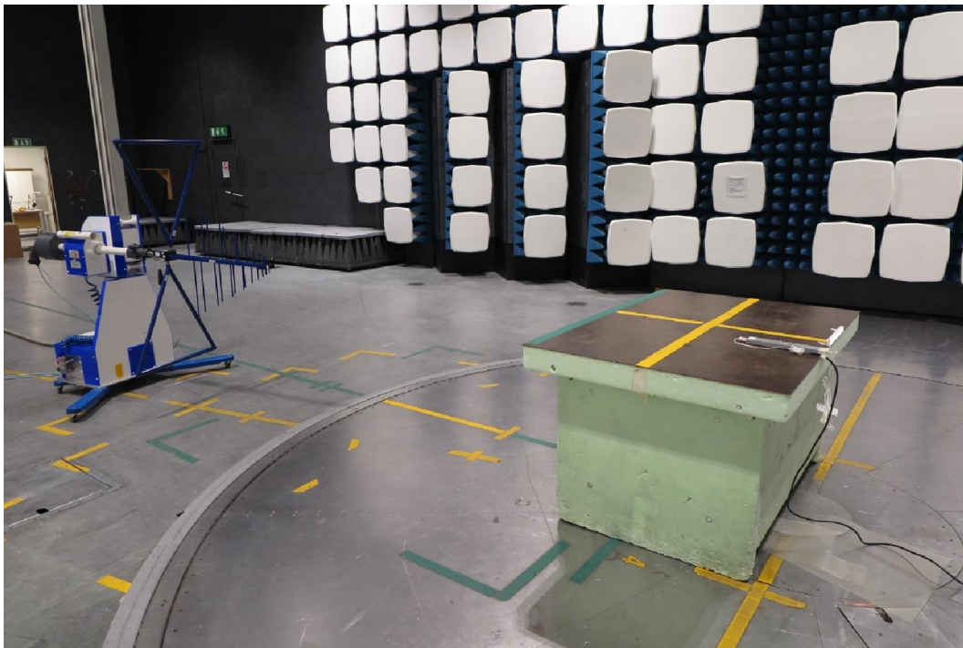
Test set up radiated emission 30 MHz – 1 GHz, with ICPSLC24-30NA-IL-1
