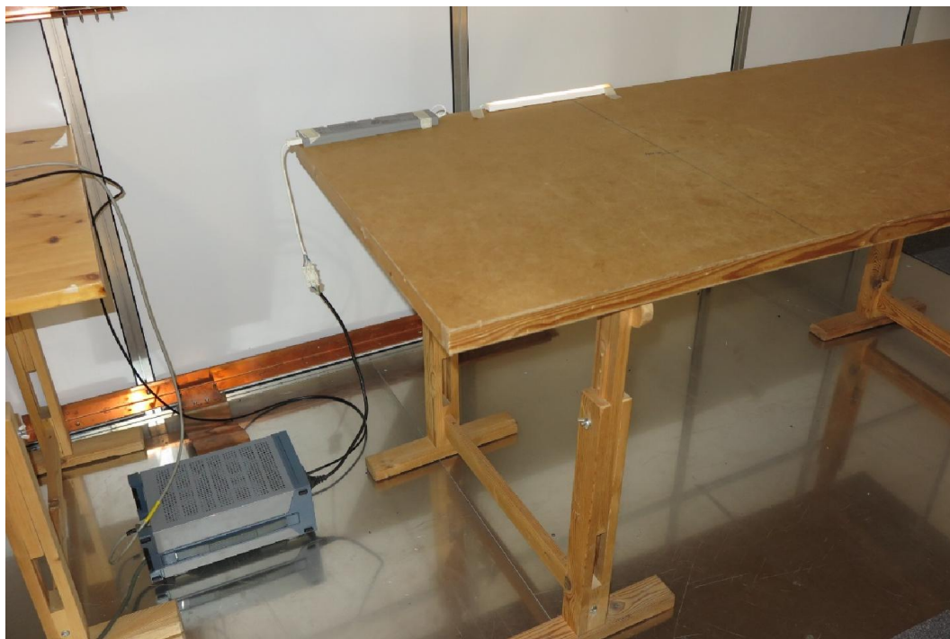
Test setup for conducted emission 150 kHz – 30 MHz, with ICPSLC24-30NA-IL-1
