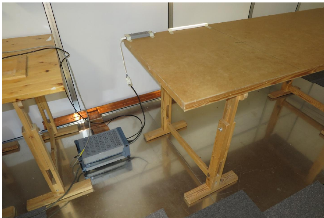
Test setup for conducted emission 150 kHz – 30 MHz, with ICPSLC24-10NA-IL-1
