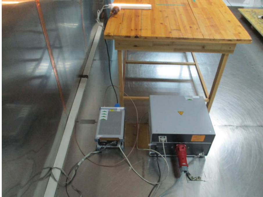
Photograph 1: Set-up for measurement of conducted emission
