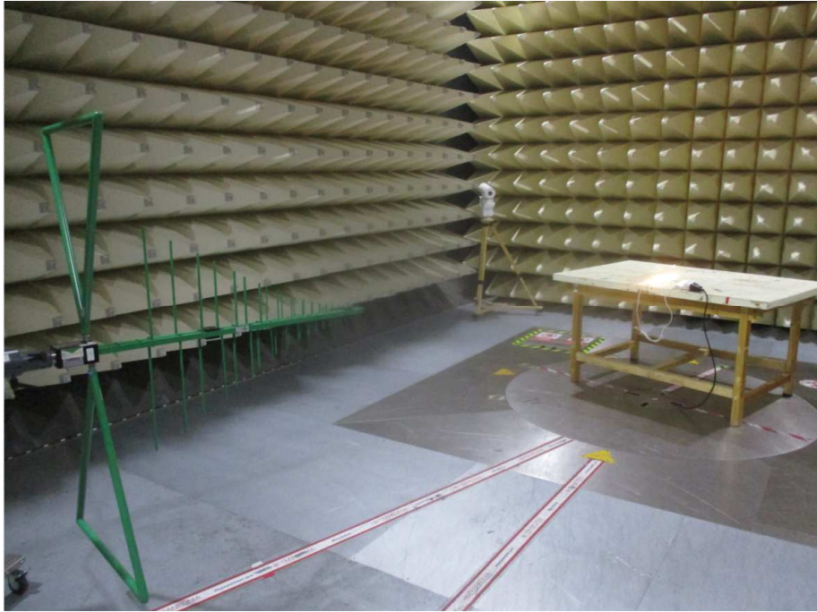
Photograph 1: Set-up for measurement of radiated emission
