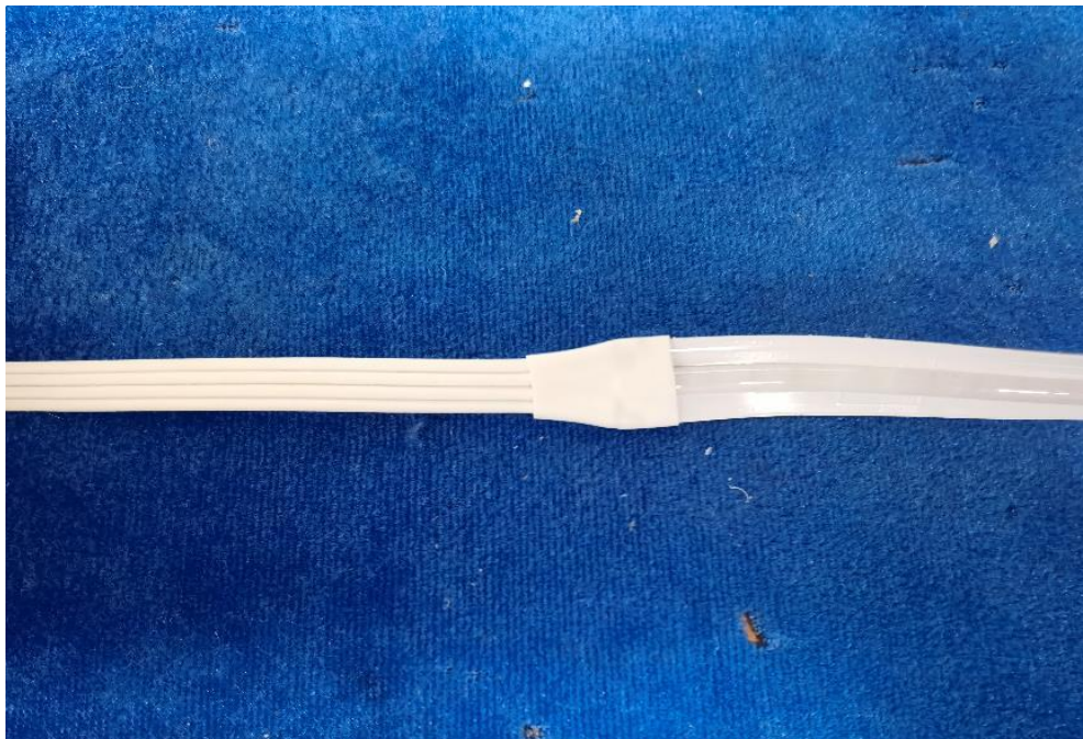
Insulation tube fix on LED module
