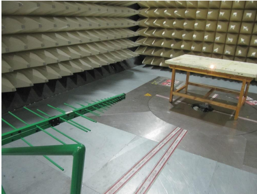
Photograph 1: Set-up for measurement of radiated emission
