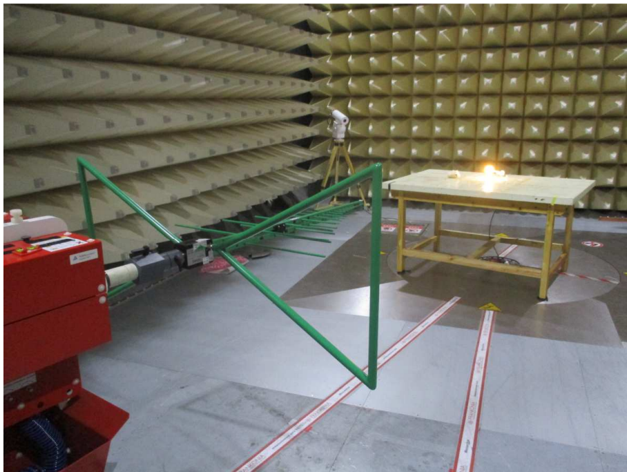
Photograph 2: Set-up for measurement of radiated emission
