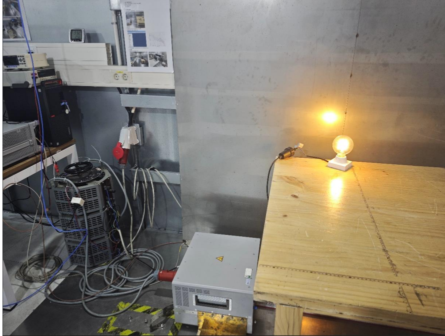
Photograph 1: Set-up for measurement of conducted emission
