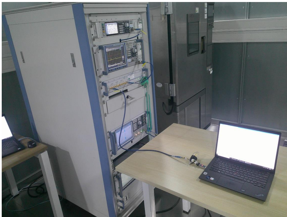
Photograph 1: Set-up photo for RF Conducted Test
