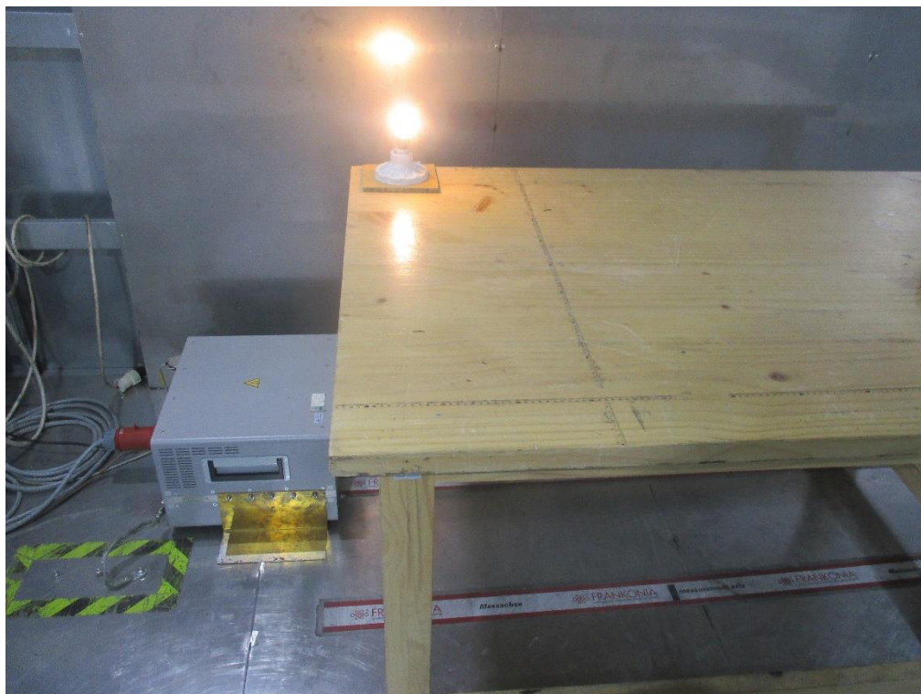
Photograph 2: Set-up photo for Conducted Emission
