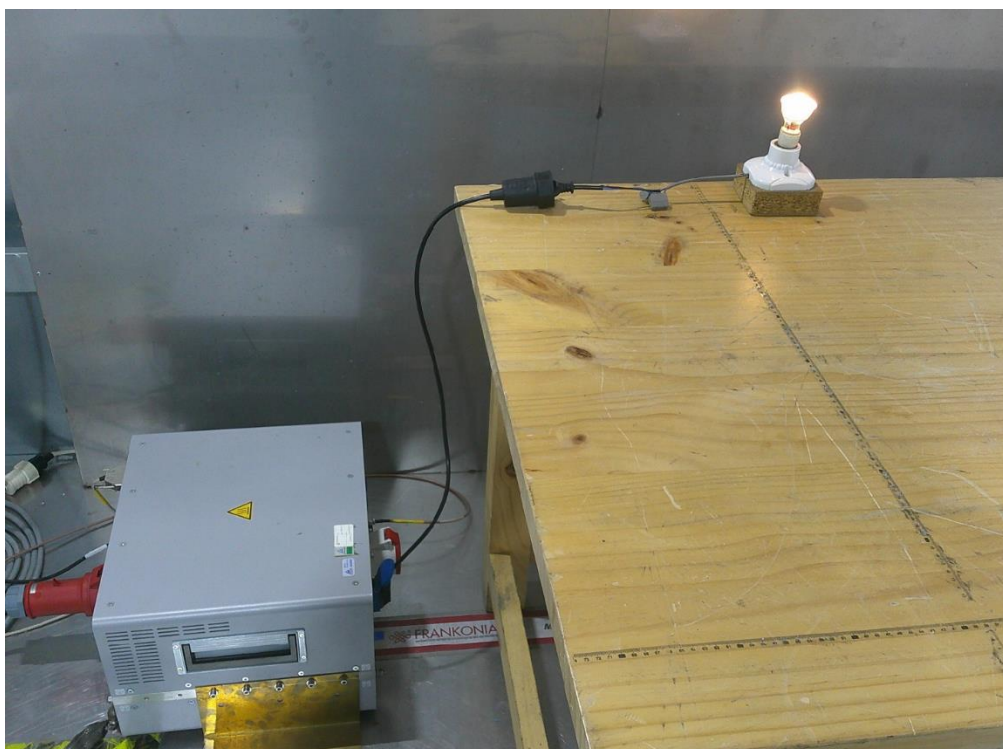
Photograph 2: Set-up photo for Conducted Emission
