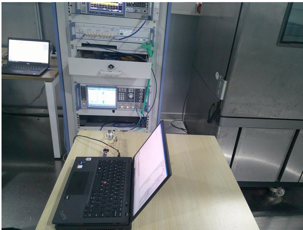
Photograph 1: Set-up photo for RF Conducted Test
