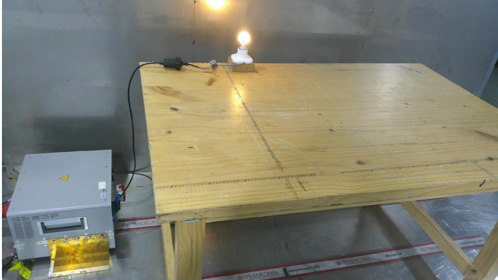
Photograph 1: Set-up for measurement of conducted emission
