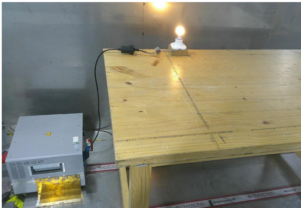
Photograph 2: Set-up photo for Conducted Emission
