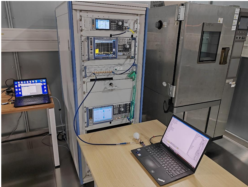
Photograph 1: Set-up photo for RF Conducted Test
