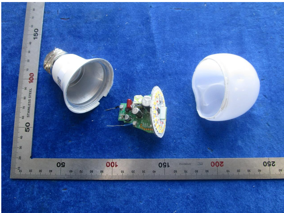
Open view (with SILABS RF IC)
