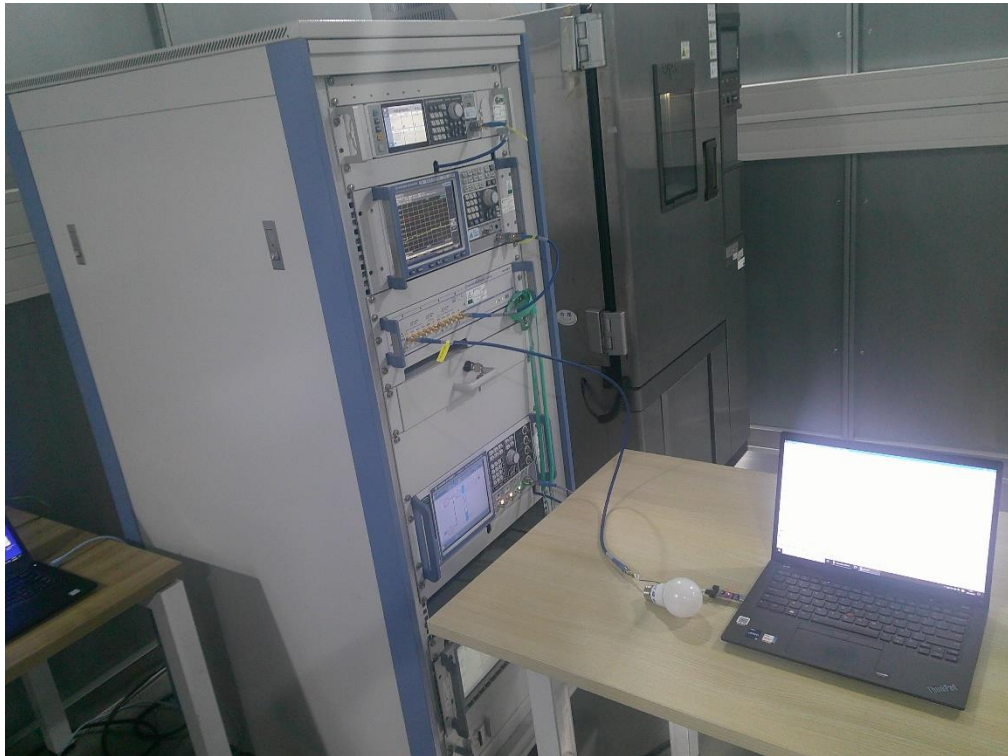
Photograph 1: Set-up photo for RF Conducted Test
