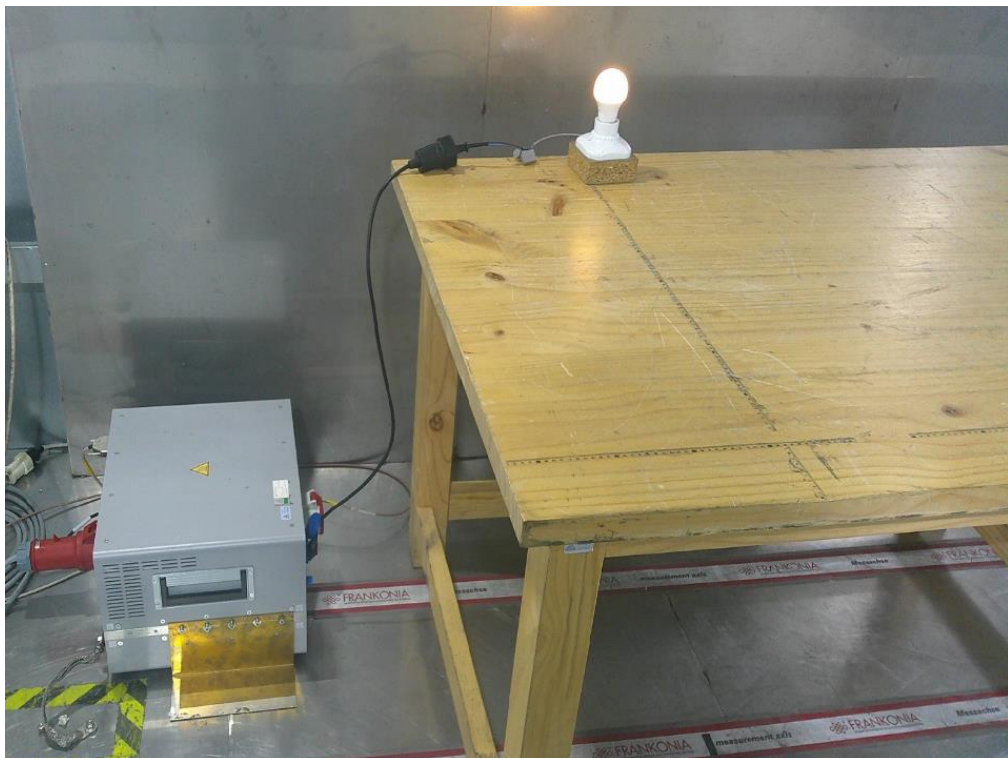
Photograph 2: Set-up photo for Conducted Emission
