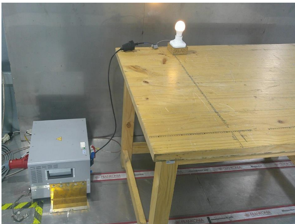
Photograph 2: Set-up photo for Conducted Emission
