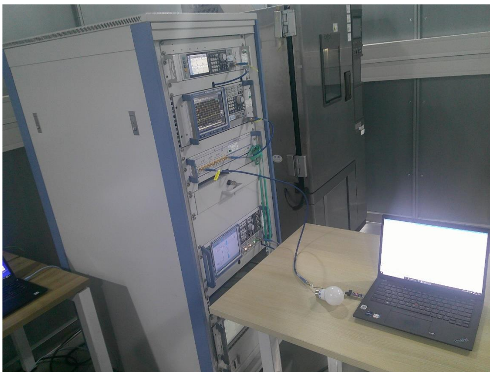
Photograph 1: Set-up photo for RF Conducted Test
