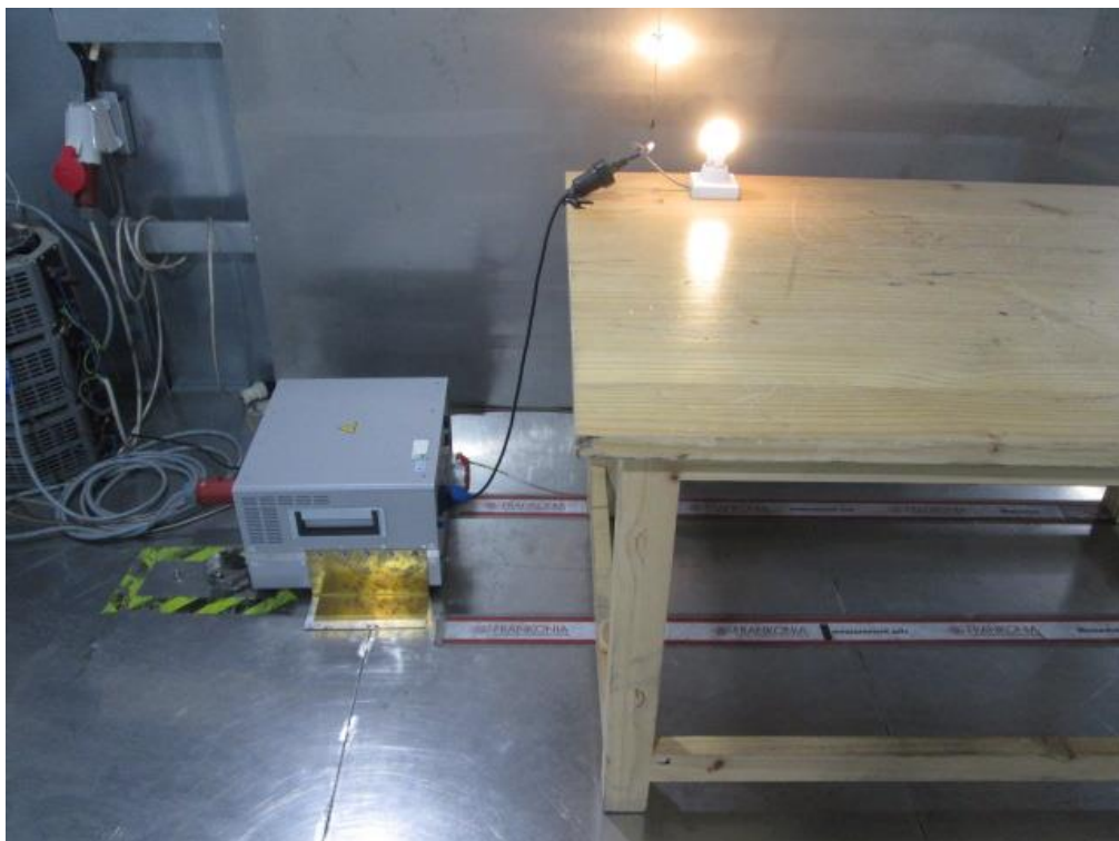
Photograph 2: Set-up photo for Conducted Emission
