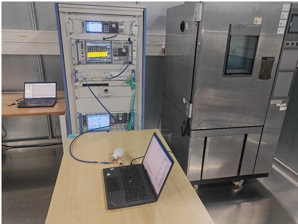
Photograph 1: Set-up photo for RF Conducted Test
