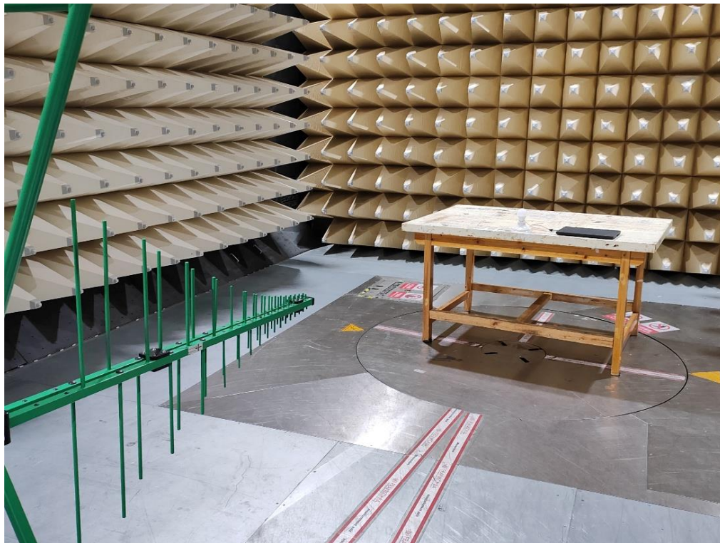
Photograph 3: Set-up photo for Radiated Emission, 30MHz - 1GHz
