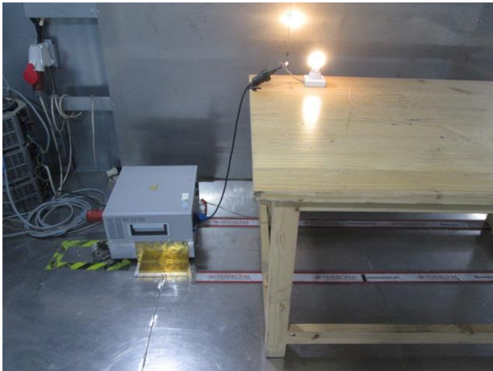
Photograph 2: Set-up photo for Conducted Emission
