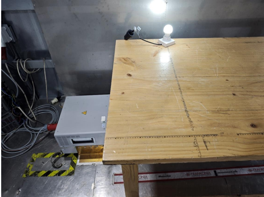
Photograph 1: Set-up for measurement of conducted emission
