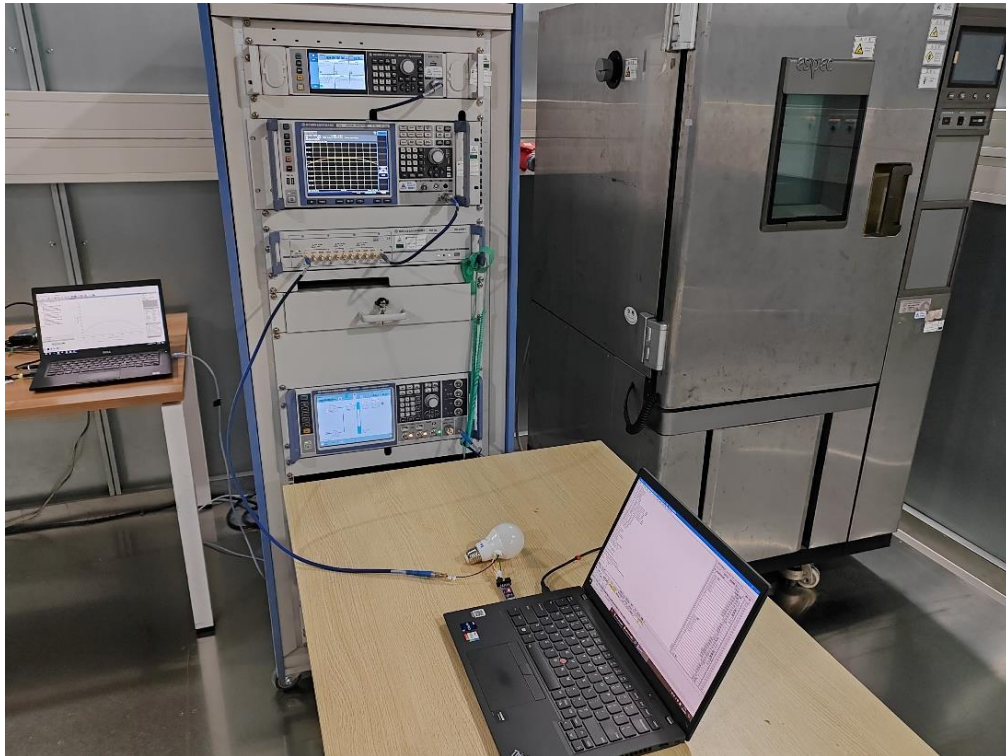
Photograph 1: Set-up photo for RF Conducted Test
