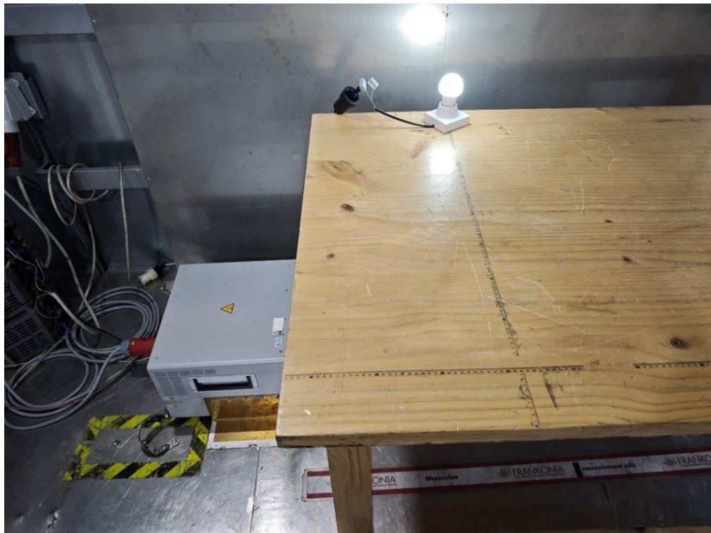
Photograph 2: Set-up photo for Conducted Emission
