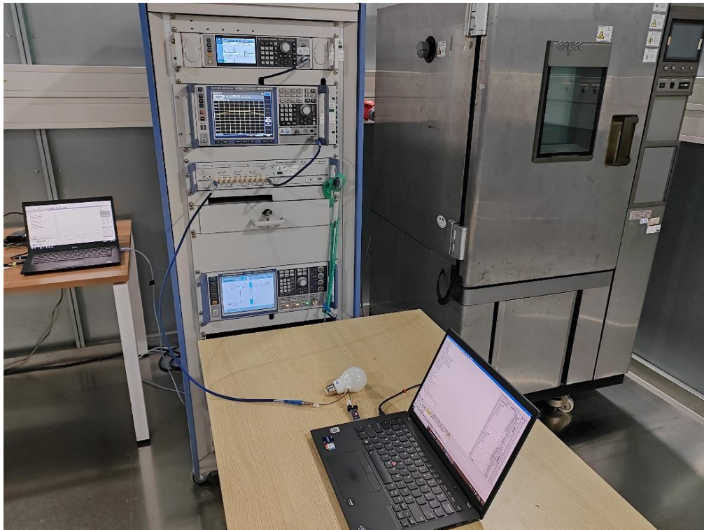
Photograph 1: Set-up photo for RF Conducted Test
