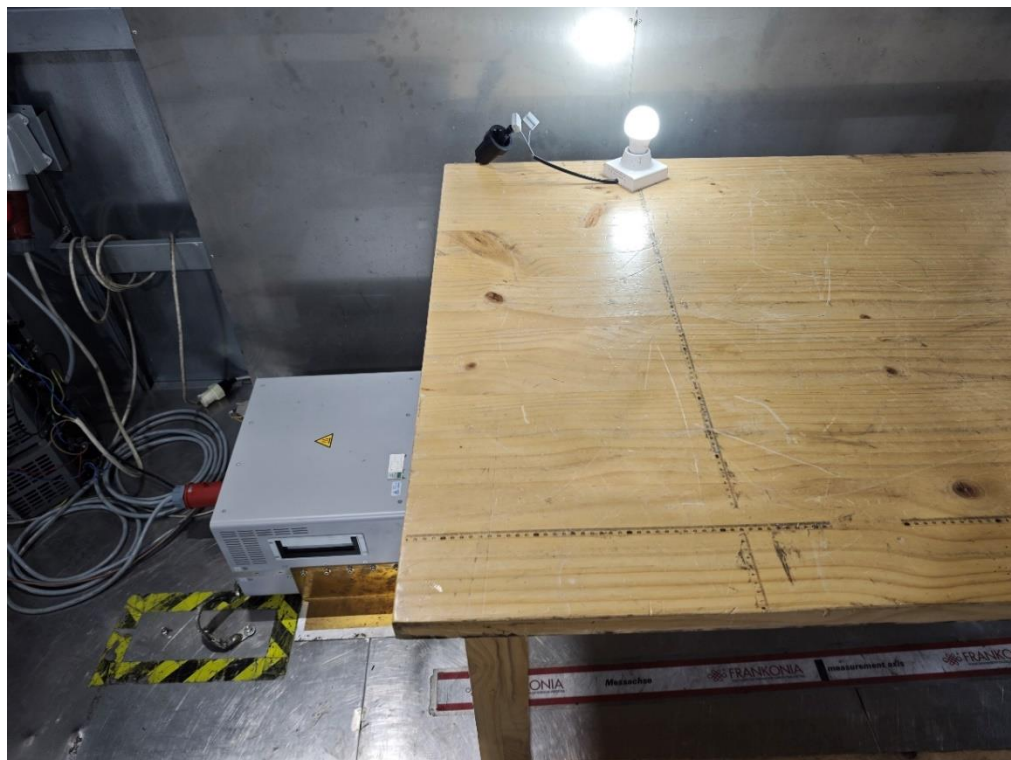
Photograph 2: Set-up photo for Conducted Emission
