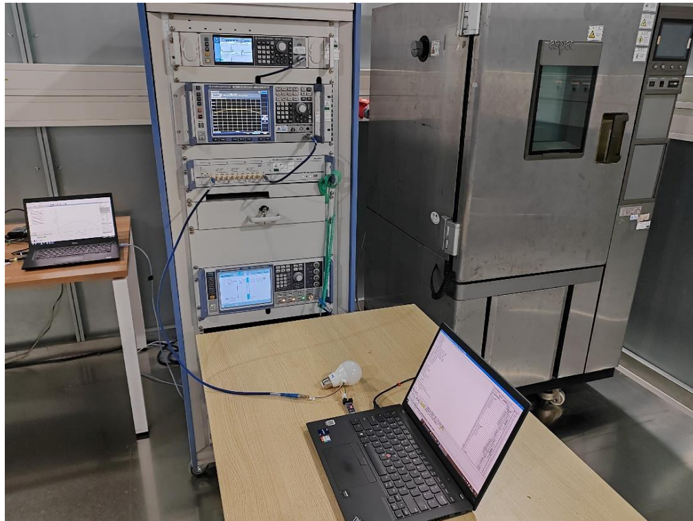
Photograph 1: Set-up photo for RF Conducted Test
