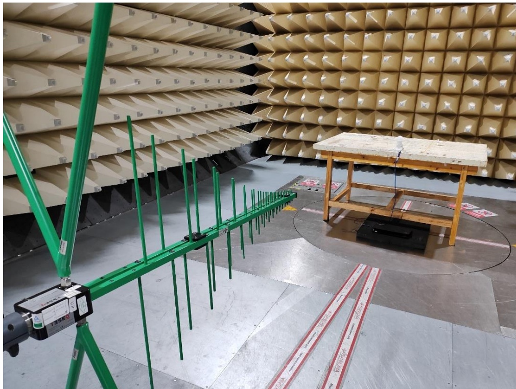
Photograph 3: Set-up photo for Radiated Emission, 30MHz - 1GHz
