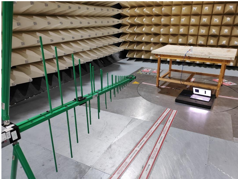
Photograph 3: Set-up photo for Radiated Emission, 30MHz - 1GHz
